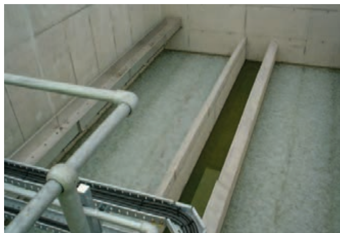
Air scour pattern test of finished filter floor (To prove level within tolerance).
